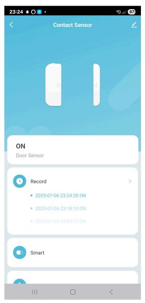
**ON/OFF**–The image in the window visually shows the current status of the device: closed contact (OFF) or open contact (ON)
