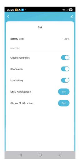
BATTERY LEVEL-Indicates the battery charge status in real time
